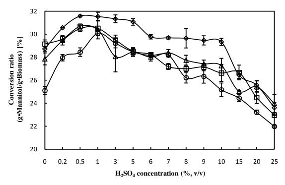
**Figure 5.** Effect of substrate and catalyst concentration on saccharification of *L. japonica*. Mannitol conversion ratio from *L. japonica* in the  $H_2SO_4$  (v/v). *L. japonica* (3% ( $\diamondsuit$ ), 5% ( $\square$ ), 7% ( $\triangle$ ) and 10% ( $\circ$ ), w/v)) was treated at 120°C by autoclaving in the  $H_2SO_4$  (v/v) range of 0 to 25%. The unit of conversion ratio is sugar obtained (g) / biomass (g)
