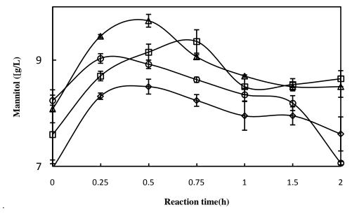
**Figure 6.** Effect of temperature (120°C ( $\diamondsuit$ ), 130°C ( $\square$ ), 140°C ( $\triangle$ ) and 150°C ( $\circ$ )) and time course on the saccharification of *L. japonica. L. japonica* (3%, w/v) was treated with 1% of H<sub>2</sub>SO<sub>4</sub> (v/v) at 0.5 MPa by hot-compress treatment instrument.
