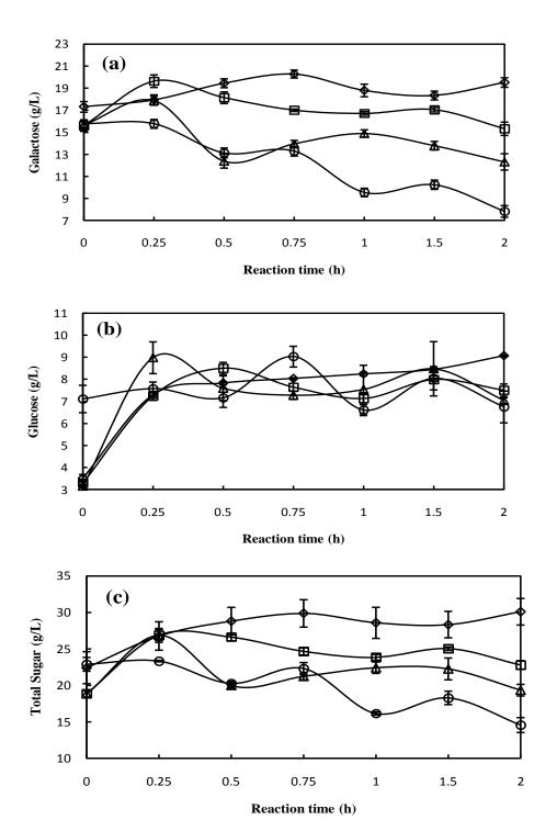
**Figure 8.** Effect of temperature (120°C ( $\diamondsuit$ ), 130°C ( $\square$ ), 140°C ( $\triangle$ ) and 150°C ( $\circ$ )) and time course on the saccharification of *G. amansii*. (a) Rhamnose (b) glucose (c) total sugar (rhamnose+glucose). *G. amansii* (3%, w/v) was treated with 3% of H<sub>2</sub>SO<sub>4</sub> (v/v) at 0.5 MPa by hot-compress treatment instrument.
