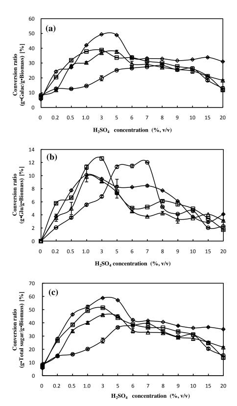
**Figure 7.** Effect of substrate and catalyst concentration on saccharification of *G. amansii*. (a) The galactose sugar conversion ratio. (b) The glucose conversion ratio. (c) The total (galactose+glucose) conversion ratio. *G. amansii* (3% ( $\diamondsuit$ ), 5% ( $\Box$ ), 7% ( $\triangle$ ), 10% ( $\circ$ ), w/v)) was treated at 120°C by autoclaving in the H<sub>2</sub>SO<sub>4</sub> (v/v) range of 0 to 25%. The unit of conversion ratio is sugar obtained (g) / biomass (g).
