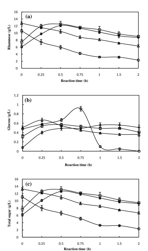
**Figure 4.** Effect of temperature (120°C ( $\diamondsuit$ ), 130°C ( $\square$ ), 140°C ( $\triangle$ ), 150°C ( $\circ$ )) and time course on the saccharification of *U. pertusa*. (a) Rhamnose (b) glucose (c) total sugar (rhamnose+glucose). *U. pertusa* (3%, w/v) was treated with 3% of H<sub>2</sub>SO<sub>4</sub> (v/v) at 0.5 MPa by hot-compress treatment instrument.
