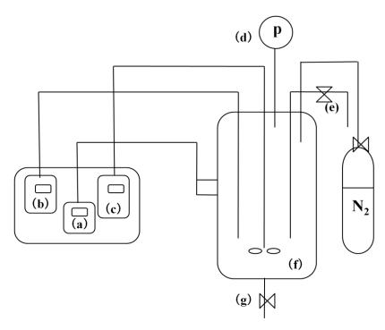
**Figure 2.** Schematic diagram of hot-compress treatment instrument: (a) Heat controller, (b) temperature controller, (c) agitator controller, (d) compressor gauge (e) sampling port, (f) 2L-reactor vessel and (g) draining port.
