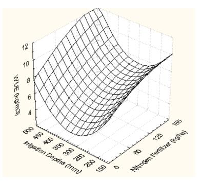
Figure 7. Relationship of irrigation depths and nitrogen fertilizer on water use efficiency (WUE).
