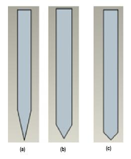
**Figure 11.** Testing cutters (a)  $\beta$ =.30°,(b)  $\beta$ =.60° and (c) $\beta$ =.90°.
