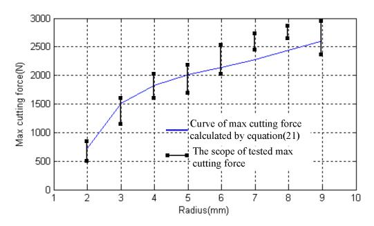
**Figure 15.** Max cutting force( $\beta = 90^{\circ}$ ).
