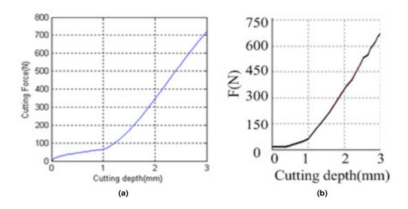
Figure 12. (a) A simulated curve and (b) a test result.
