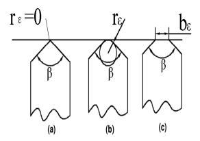
Figure 3. The shape of cut edge
