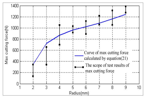
**Figure 13.** Max cutting force( $\beta$ =.30°).
