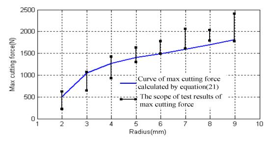
**Figure 14.** Max cutting force( $\beta$ = 60°).
