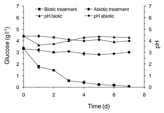
**Figure 6.** Consumption of glucose and pH in the air bubble column reactor (8 day, 30 °C, air flow: 500 cc·min<sup>-1</sup>, non-sterilized conditions).
