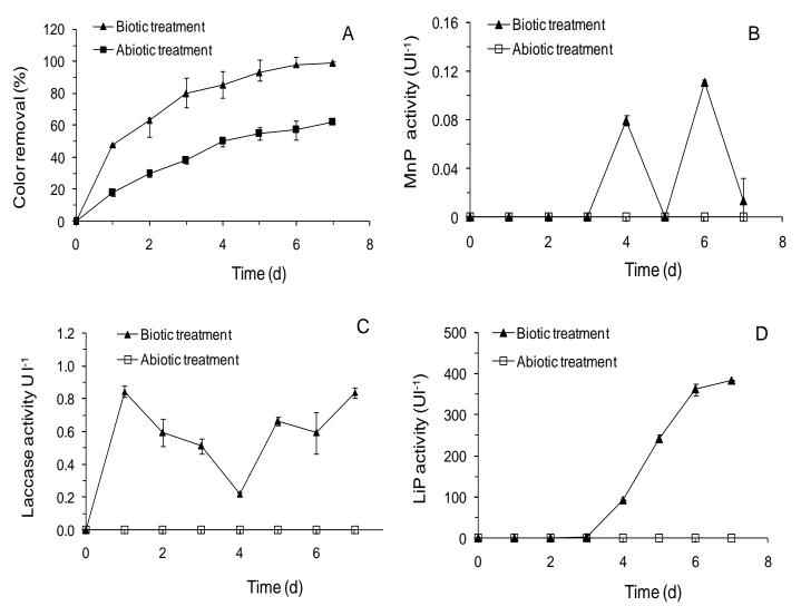
Figure 5. Removal kinetics in bubble column reactor. (A) Color removal; (B) MnP activity; (C) laccase activity; (D) LiP activity, 8 day, 30°C, air flow of 500 cc·min<sup>-1</sup> in non-sterilized conditions.
