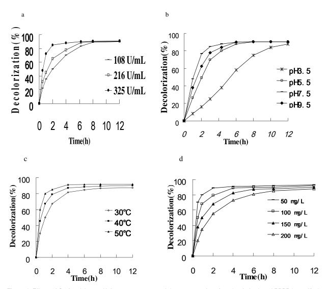
**Figure 6.** Effects of CotA activity; **a**, pH; **b**, temperature; **c** and dye concentration; **d** on decolorization of RBBR by purified CotA laccase; **a** RBBR (50 mg/L), CotA (108 to 325 U/ml), pH 7.5, 40 °C; **b** RBBR (50 mg/L), CotA (325 U/ml), pH (3.5 to 9.5), 40 °C; **c** RBBR (50 mg/L), CotA (325 U/ml), pH 7.5, 30 to 60 °C. **d** RBBR (50 to 200 mg/L), CotA (325 U/ml), pH 7.5, 40 °C.
