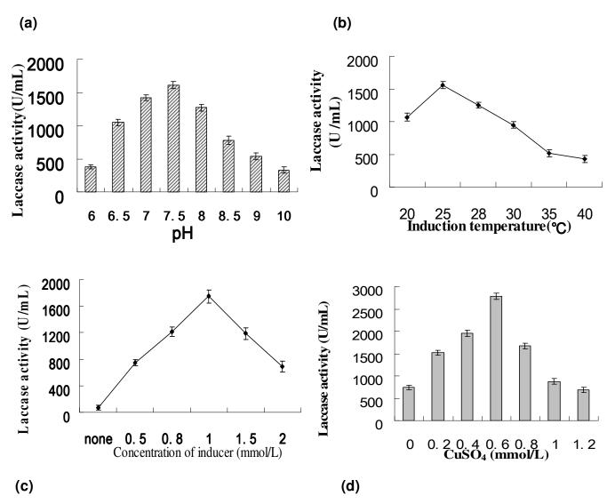
**Figure 2.** Effects of pH; **a** Induce temperature; **b** IPTG concentration; **c** and copper concentration; **d** on the production of laccase in LB medium supplemented with 0.2 mmol/L CuSO<sub>4</sub>. Cultivation conditions; **a** 0.2 mmol/L CuSO<sub>4</sub>, 1 mmol/L IPTG, 30°C; **b** 0.2 mmol/L CuSO<sub>4</sub>, pH 7, 30°C; **c** 0.2 mmol/L CuSO<sub>4</sub>, 1 mmol/L IPTG, 30°C; **d** 1 mmol/L IPTG, pH 7, 30°C.
