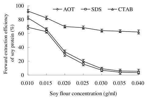
**Figure 1.** Effects of soy flour concentrations on the forward extraction efficiency of soy protein using different reverse micelle systems. Extraction conditions were as follows: Wo 16, pH 6.5 for AOT and SDS, and pH 10 for CTAB, temperature 35℃, extraction time 20 min, KCI concentration 0.1 mol/L, ultrasound power 240 W for AOT, 210 W for SDS and 270 W for CTAB.
