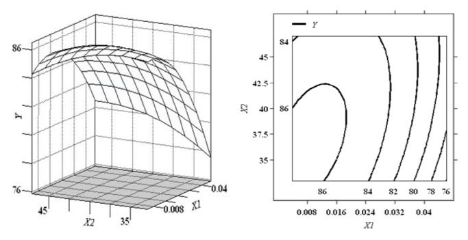
**Figure 8.** Response surface and contour plots for the effects of soy flour concentration ( $X_1$ ) and temperature ( $X_2$ ) on forward extraction efficiency of soy protein (Y) at pH 7.
