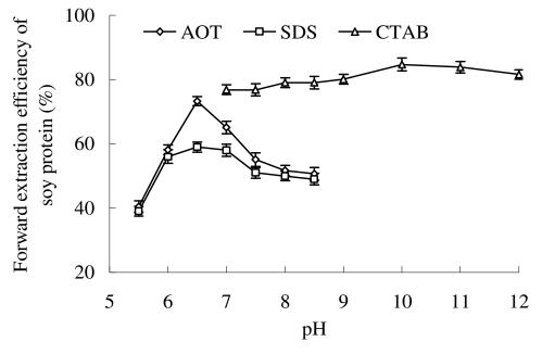
**Figure 6.** Effects of pH on forward extraction efficiency of soy protein using different reverse micelle systems. Extraction conditions were as follows: soy flour concentration 0.01 g/ml, Wo 16, temperature 35 °C; extraction time 20 min; KCI concentration 0.1 mol/L; ultrasound power 240 W for AOT; 210W for SDS and 270 W for CTAB
