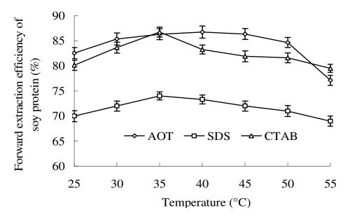
**Figure 4.** Effects of temperature on forward extraction efficiency of soy protein using different reverse micelle systems. Extraction conditions were as follows: soy flour concentration 0.01 g/ml, Wo 16, pH 6.5 for AOT and SDS, and pH 10 for CTAB, extraction time 20 min, KCI concentration 0.1 mol/L; ultrasound power 240 W for AOT, 210 W for SDS and 270 W for CTAB.
