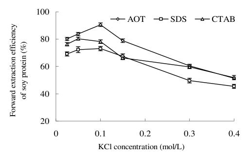
Figure 5. Effects of KCI concentration on forward extraction efficiency of soy protein using different reverse micelle systems. Extraction conditions were as follows: Soy flour concentration 0.01 g/ml, Wo 16, pH 6.5 for AOT and SDS, and pH 10 for CTAB, temperature 35 ℃, extraction time 20 min, ultrasound power 240 W for AOT, 210 W for SDS and 270 W for CTAB.
