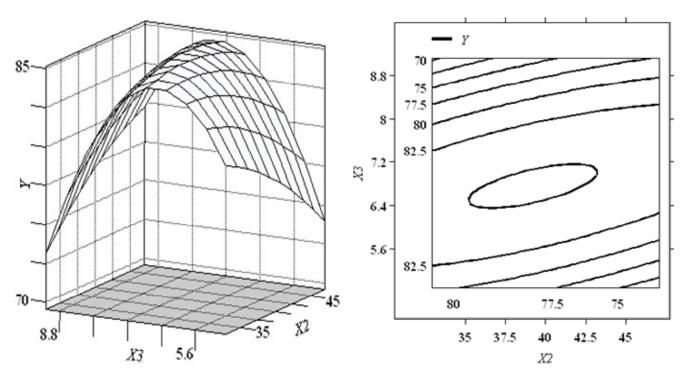
**Figure 10.** Response surface and contour plots for the effects of temperature ( $X_2$ ) and pH ( $X_3$ ) on forward extraction efficiency of soy protein (Y) at soy flour concentration 0.025 g/ml.
