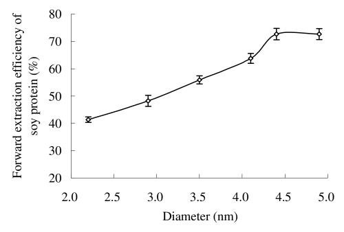
Figure 11. Effects of diameter of AOT reverse micelle on forward extraction efficiency of soy protein.
