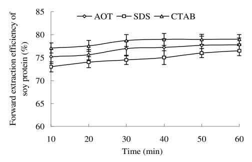
**Figure 3.** Effects of extraction time on forward extraction efficiency of soy protein using different reverse micelle systems. Extraction conditions were as follows: soy flour concentration 0.01 g/ml, Wo 16, pH 6.5 for AOT and SDS, and pH 10 for CTAB, temperature 35 ℃, KCl concentration 0.1 mol/L; ultrasound power 240 W for AOT, 210 W for SDS and 270 W for CTAB.
