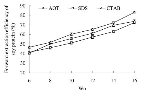
**Figure 2.** Effects of Wo on forward extraction efficiency of soy protein using different reverse micelle systems. Extraction conditions were as follows: soy flour concentration 0.01 g/ml, pH 6.5 for AOT and SDS, and pH 10 for CTAB, temperature 35 °C, extraction time 20 min, KCI concentration 0.1 mol/L; ultrasound power 240 W for AOT, 210 W for SDS and 270 W for CTAB.
