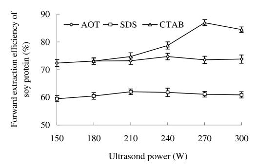
**Figure 7.** Effects of ultrasound power on forward extraction efficiency of soy protein using different reverse micelle systems. Extraction conditions were as follows: soy flour concentration 0.01 g/ml, Wo 16; pH 6.5 for AOT and SDS, and pH 10 for CTAB; temperature 35°C; extraction time 20 min; KCI concentration 0.1 mol/L.
