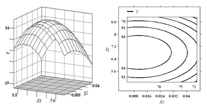
**Figure 9.** Response surface and contour plots for the effects of soy flour concentration ( $X_1$ ) and pH ( $X_3$ ) on forward extraction efficiency of soy protein (Y) at a temperature of 40 °C.
