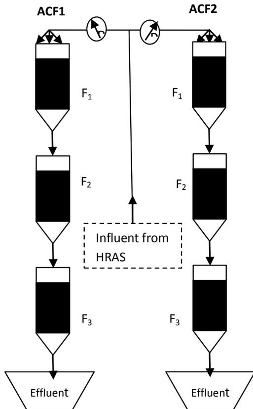
**Figure 3.** Schematic representation of the setup of the alternating charcoal filter 1 (ACF1) with a retention time of 2.5 h and the alternating charcoal filters 2 (ACF2) with a retention time of 5 h.
