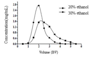
Figure 3. Elution curves of CA with two concentration of ethanol (left).
