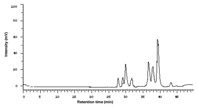
Figure 2. Standard fatty acid mixture chromatogram.
