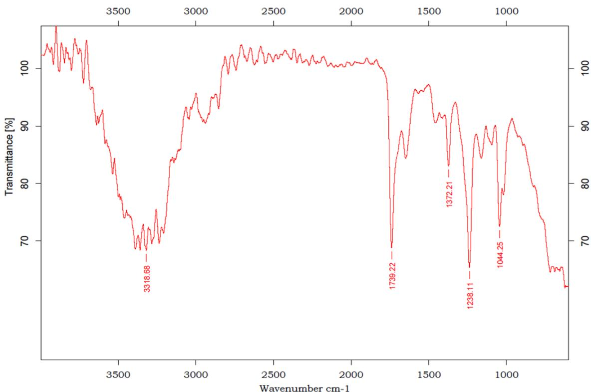
**Figure 8.** FTIR spectrum of transesterified olive oil. The *n*-hexane extracted products were used for spectral analysis which were obtained by incubating the purified enzyme with olive oil and methanol at 30°C with shaking at 150 rpm for 48 h followed by extraction with *n*-hexane.
