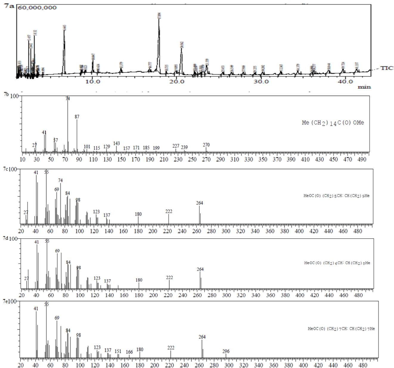
**Figure 7.** FAME's (Biodiesel) production using purified lipase from *Emericella nidulans*. **a**, Full scan GC-MS chromatogram of FAME's synthesized by incubating purified lipase with olive oil and methanol at 30°C with shaking at 150 rpm for 48 h followed by extraction of products (methyl esters) with n-hexane. **b**, mass spectra of hexadecanoic acid ethyl ester. **c**, 7-octadecenoic acid methyl ester. **d**, 8-octadecenoic acid methyl ester. **e**, 9-octadecenoic acid methyl ester.
