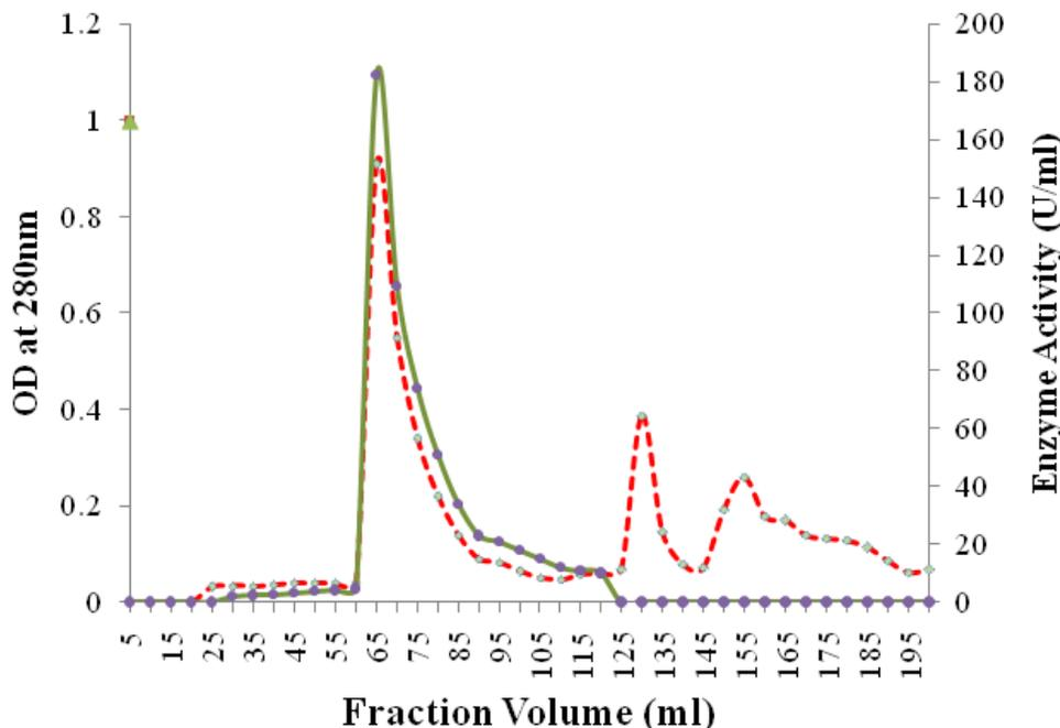
**Figure 2.** Elution profile of Enzyme fractions obtained from HIC using Phenyl sepharose. Elution of proteins from the column was followed by measuring absorbance at 280 nm using UV absorbance at 280 nm and by spectro photometric estimation of the enzyme activity using pNP-palmitate as substrate.
