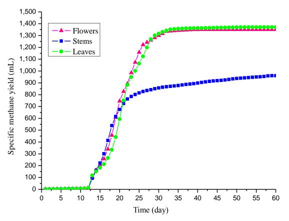
Figure 2. The specific methane yield of the three samples of BSW.
