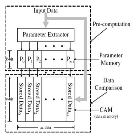
Figure 3. Pre-computation block of CAM.
