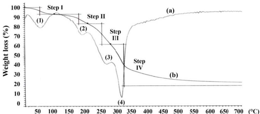
**Figure 2.** The thermal gravimetric analyzer (TG/DTA) curve (a) and TG curve (b) show typical weight losses of components in raw pineapple peel monitored in the range of 30–830 °C. Step I: moisture removal (I), Step II: hemicellulose degradation (II), Step III: cellulose degradation (III) and Step IV: lignin degradation (4).
