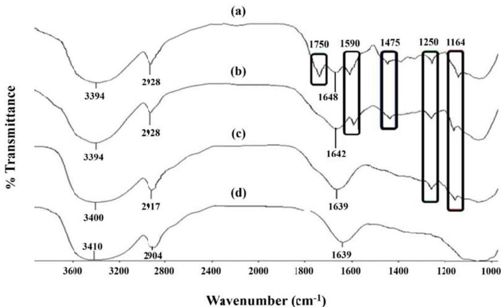
**Figure 1.** The IR spectra of (a) raw pineapple peel, (b) Sample I = lignin + hemicellulose + cellulose, (c) Sample II = hemicellulose + cellulose and (d) Sample III = cellulose. The mode assignment of the functional groups in each main component was removed.
