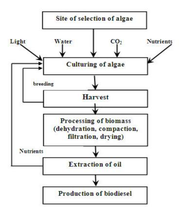
Figure 2. The stages of biodiesel production from microalgae.
