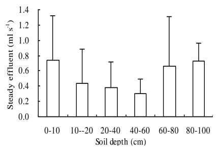
Figure 3. Variation of steady effluent at different soil depths; the bar is the standard errors.
