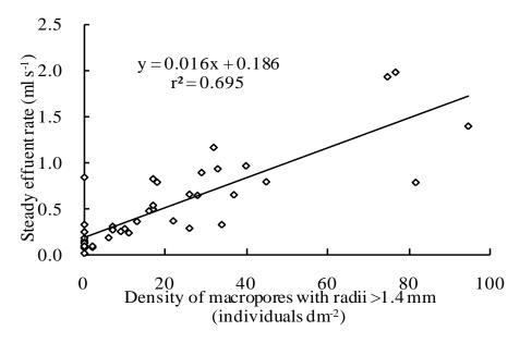
Figure 7. Effect of the densities of macropores with radii > 1.4 mm on the steady effluent rates.
