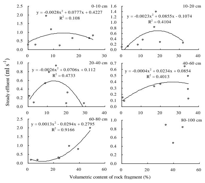
Figure 10. Effect of volumetric content of rock fragments on the water steady effluent volume.
