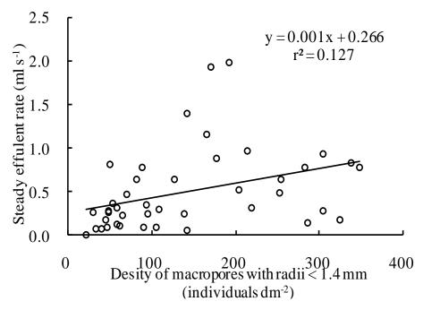
Figure 8. Effect of the densities of macropores with radii < 1.4 mm on the steady effluent rates.
