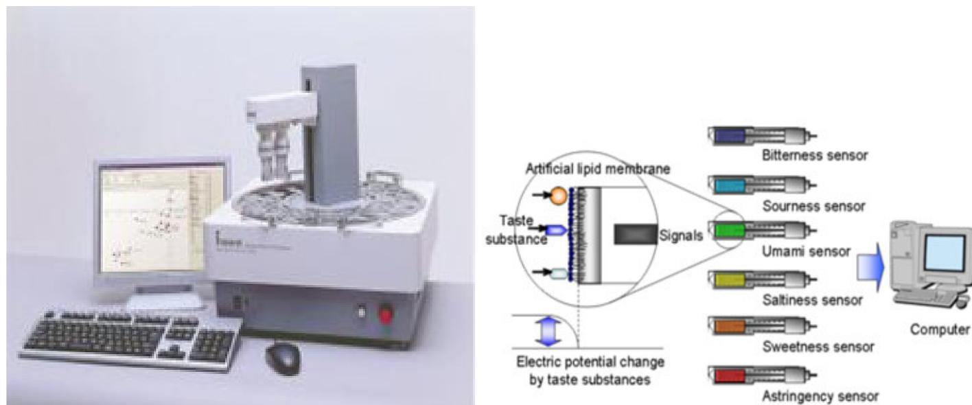
**Figure 1.** ET apparatus and the taste sensors (taste sensing system SA402B).
