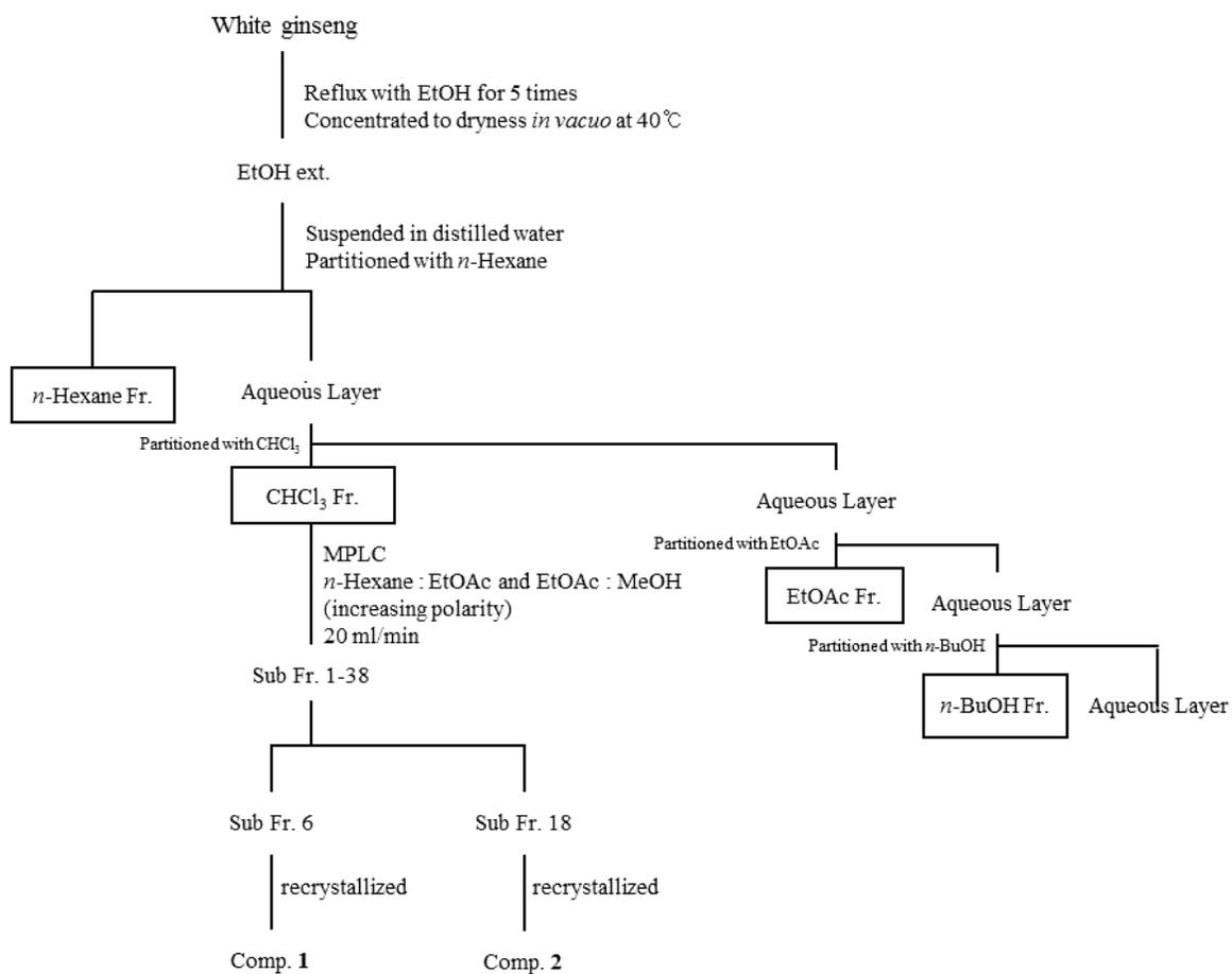
**Figure 4.** Fractionation and isolation scheme for compounds 1 and 2.
