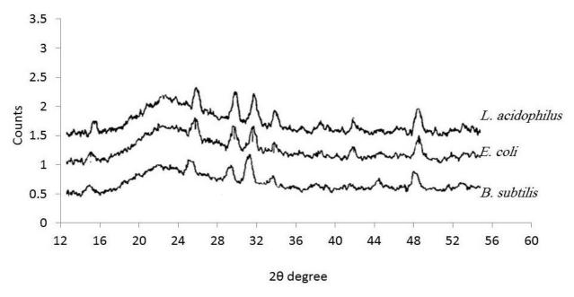
Figure 1. X-ray diffraction patterns of CdS nanoparticles prepared by E. coli, L. acidophilus and B. Subtilis at room temperature.
