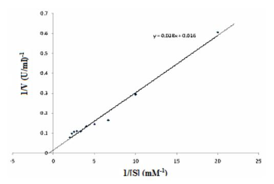
**Figure 5a.** Lineweaver-Burk plot (1/V versus 1/[S]) for the determination of kinetic parameters of the rhodanese of *P. aeruginosa*. Enzyme was assayed at varying concentrations of KCN at 50 mM  $Na_2S_2O_3$ .
