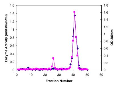
**Figure 2a.** Elution profile of rhodanese of *P. aeruginosa* on CM Sepharose CL-6B. The column was equilibriated with 200 ml of 50 mM citrate buffer, pH 5.0 and then eluted with 250 ml linear gradient of 0-0.5 M KCl in 50 nM citrate buffer, pH 5.0. Fractions of 3 ml were collected at a flow rate of 36 ml/h. -+-+, Enzyme activity; -=-=-, protein profile.
