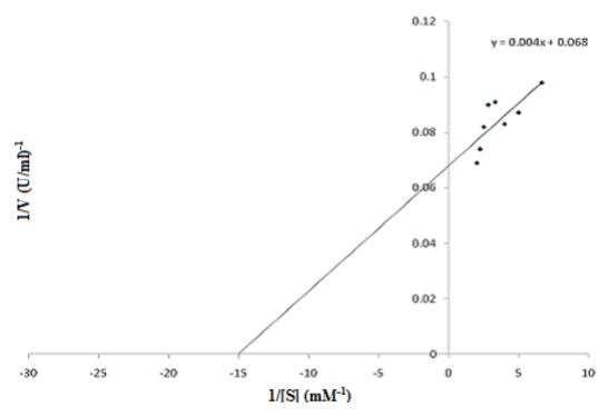
**Figure 5b.** Lineweaver-Burk plot (1/V versus 1/[S]) for the determination of kinetic parameters of the rhodanese of *P. aeruginosa*. Enzyme was assayed at varying concentrations of Na<sub>2</sub>S<sub>2</sub>O<sub>3</sub> at 50 mM KCN.
