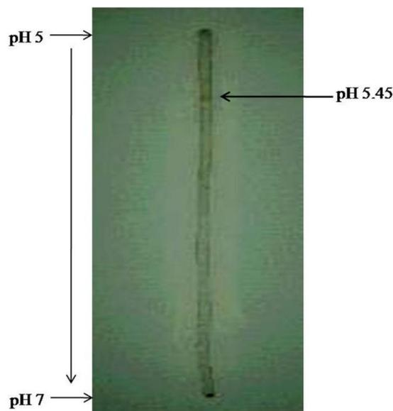
**Figure 3.** The isoelectric point (pI) of chitosanase. It was measured using isoelectric focusing on 5% polyacrylamide gel slab containing 2% carrier ampholyte of pH 5 to 7.
