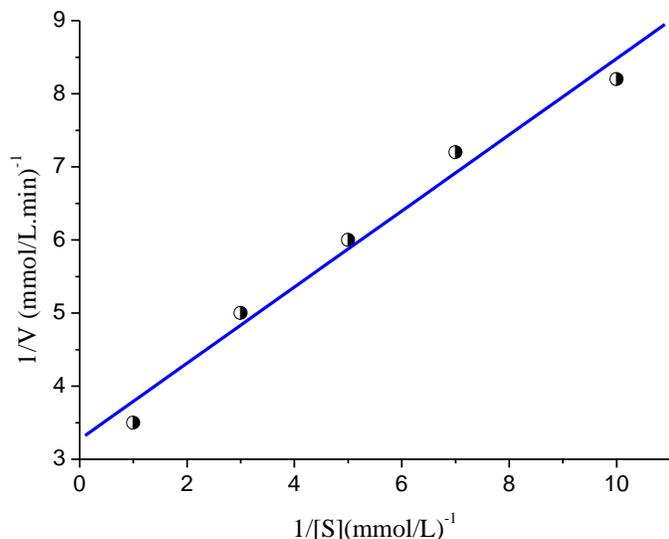
**Figure 4.** Kinetic parameter determination from Lineweaver–Burk plot. Enzyme activities were measured at 40°C by incubating chitosan with chitosanase in 0.5 M NaOH.
