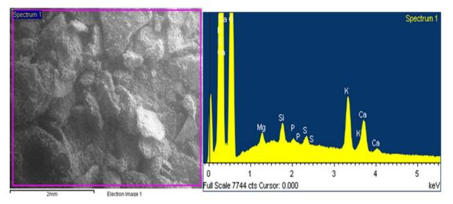
Figure 1a. Mineral analysis as determined by energy dispersive X-ray spectroscopy (EDX).
