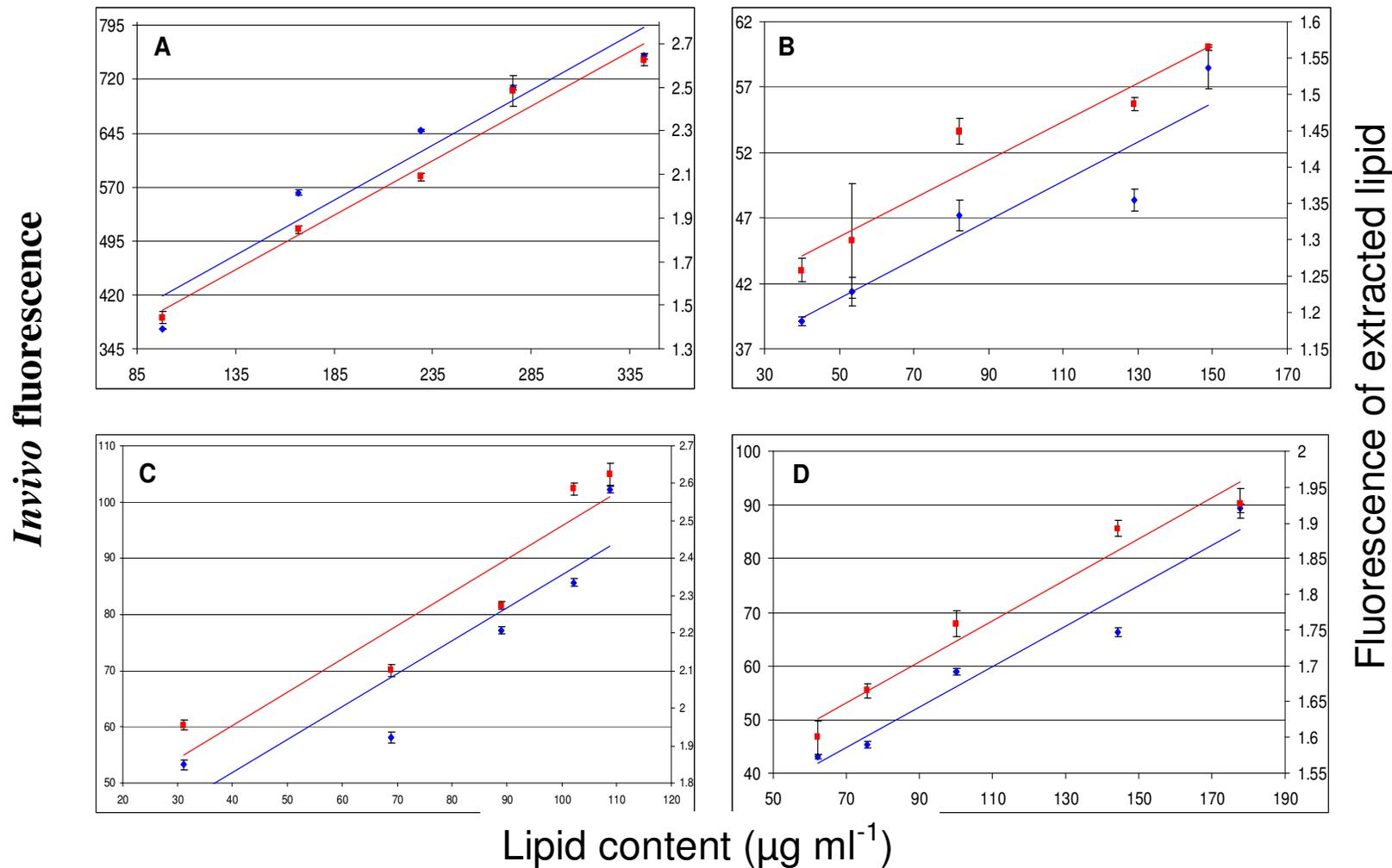
**Figure 3.** Relationship of *in vivo* fluorescence (♦) and fluorescence intensity of the extracted lipid (■) to the gravimetrically determined lipid content of (A) *Isochrysis galbana*, (B) *Tetraselmis* sp., (C) *Alexandrium minutum* and (D) *Prorocentrum lima* after Nile red staining.
