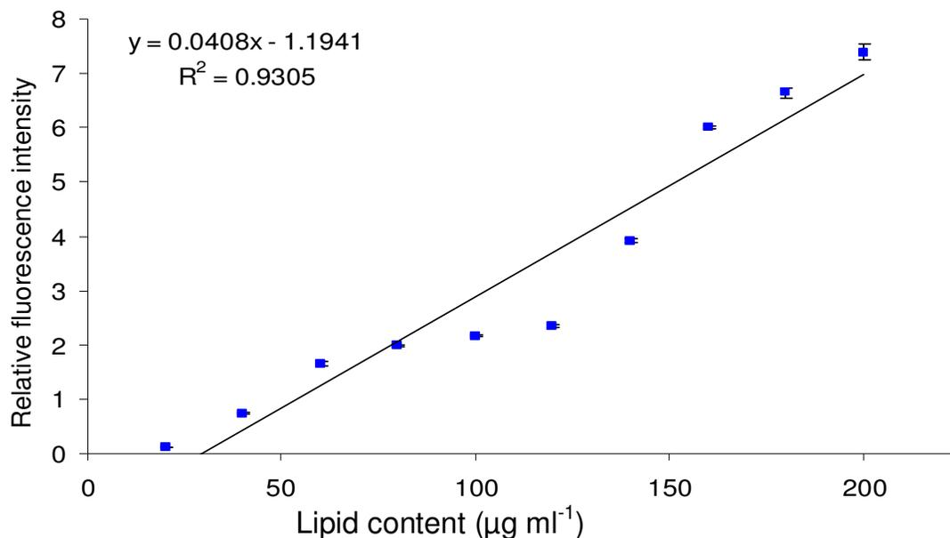
**Figure 5.** Relative fluorescence intensity (♦) of different concentrations of commercial oil after Nile red staining. The fluorescence intensity was obtained from the difference between the fluorescence of the sample and the fluorescence of Nile red alone.
