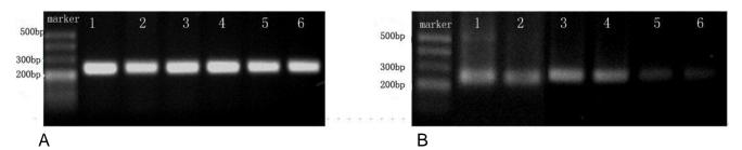
Figure 1. Comparison of two methods in agarose gel electrophoresis. A, Precasting gels method. B, staining sample method.
