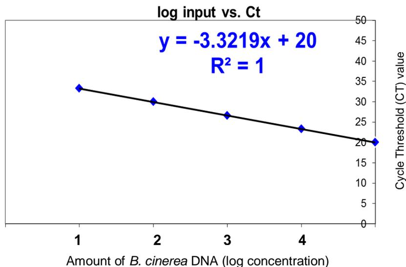
**Figure 3.** Standard curve generated from the amplification of 10-fold dilutions of internal control (actin). This curve revealed a good linear relationship ( $R^2 = 1$ ) between the  $\log_{10}$  value of the starting cell concentration and the threshold.
