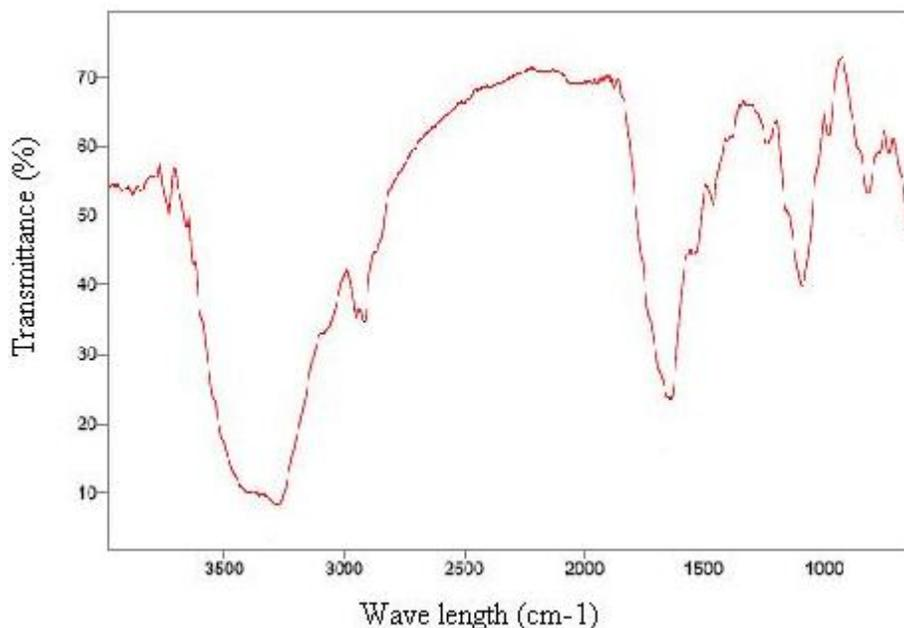
**Figure 5.** The IR spectrum of the partially purified microbial demulsifier produced by *Microbacterium* sp.
