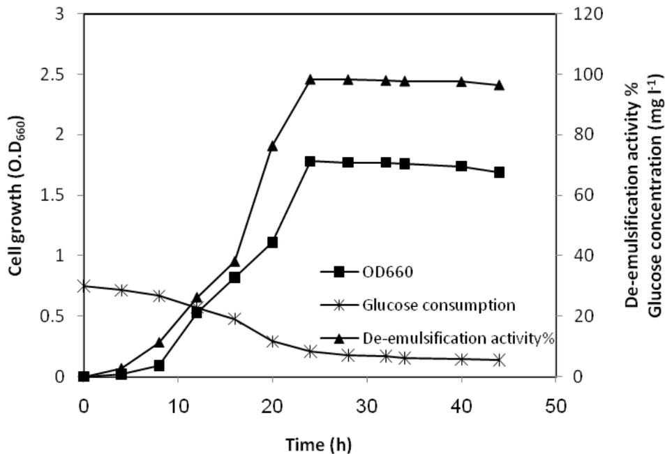
**Figure 3.** The cell growth, glucose consumption, demulsification activity of *Microbacterium* in a 5 L fermenter at 25°C, 200 rpm, and 0.5 vvm. Glucose: 30 g L<sup>-1</sup>, yeast extract: 1.0 g L<sup>-1</sup>.
