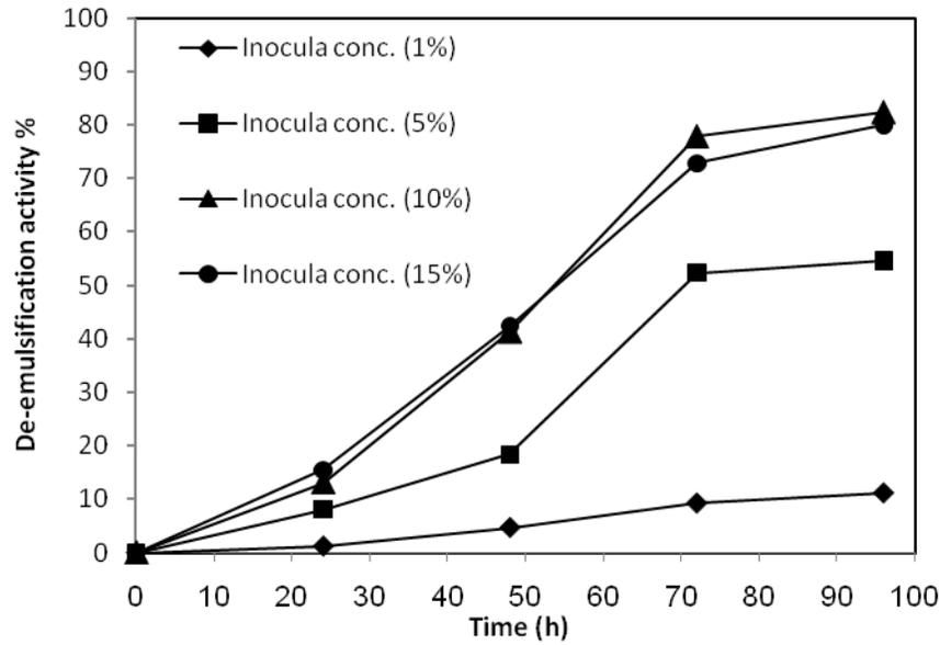
**Figure 2.** Effect of inoculum concentration on the demulsification of the model emulsion by *Microbacterium* culture under unoptimized production. Bacterial counts was  $5 \times 10^8$  CFU mL<sup>-1</sup>. W/CO demulsification assay temperature was 80 °C for 48 h. Control experiment carried out by adding uninoculated medium was negligible.
