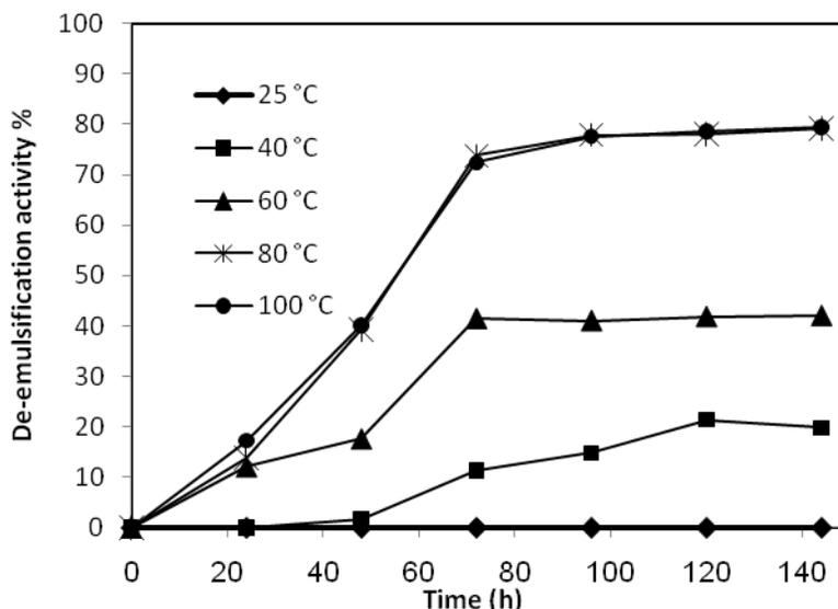
**Figure 1.** Effect of W/CO demulsification assay temperature on demulsifying the model emulsion by *Microbacterium* culture under unoptimized production. Inoculum concentration was 10% v/v (bacterial counts:  $5 \times 10^8$  CFU mL<sup>-1</sup>). Cultivation temperature was 30°C. W/CO demulsification assay time was 48 h. Control experiment carried out by adding uninoculated production medium was negligible.
