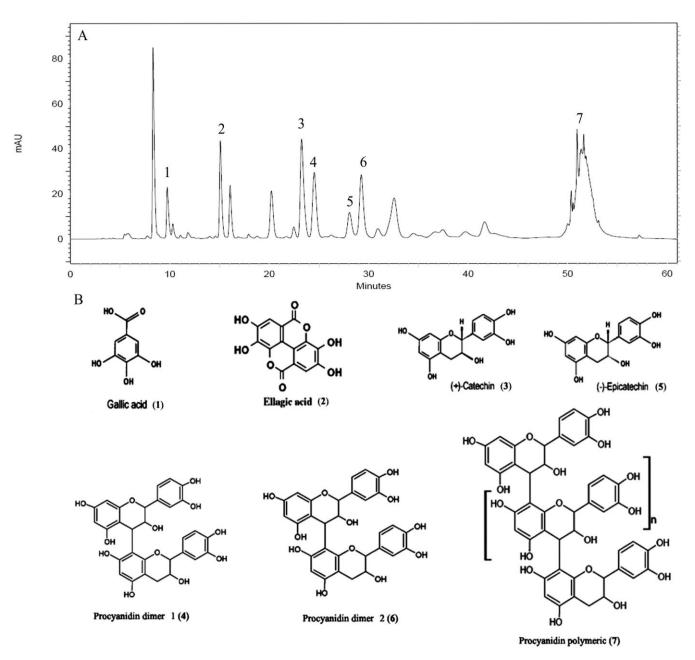
Figure 2. A) HPLC trace of ethyl acetate fraction at 280 nm. Captions: gallic acid (1), ellagic acid (2), catechin (3), procyanidin dimer 1 (4), epicathechin (5), procyanidin dimer 2 (6) and polymeric procyanidin (7) were obtained; B) Structures of substances identified in the ethyl acetate fraction of *C. nucifera* L. aqueous husk fiber extract.
