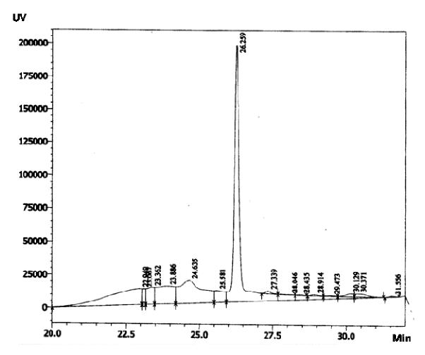
Figure 2. HPLC chromatogram of OTA standard. Retention time (RT): 26.259.
