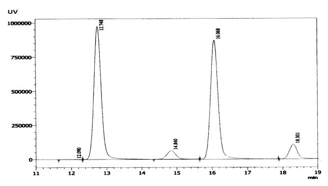
Figure 1. HPLC chromatogram of aflatoxin standards. Retention time (RT), 12.748; aflatoxin G2, RT 14.84; aflatoxin G1, RT 16.068; aflatoxin B2 and RT 18.301, aflatoxin B1.
