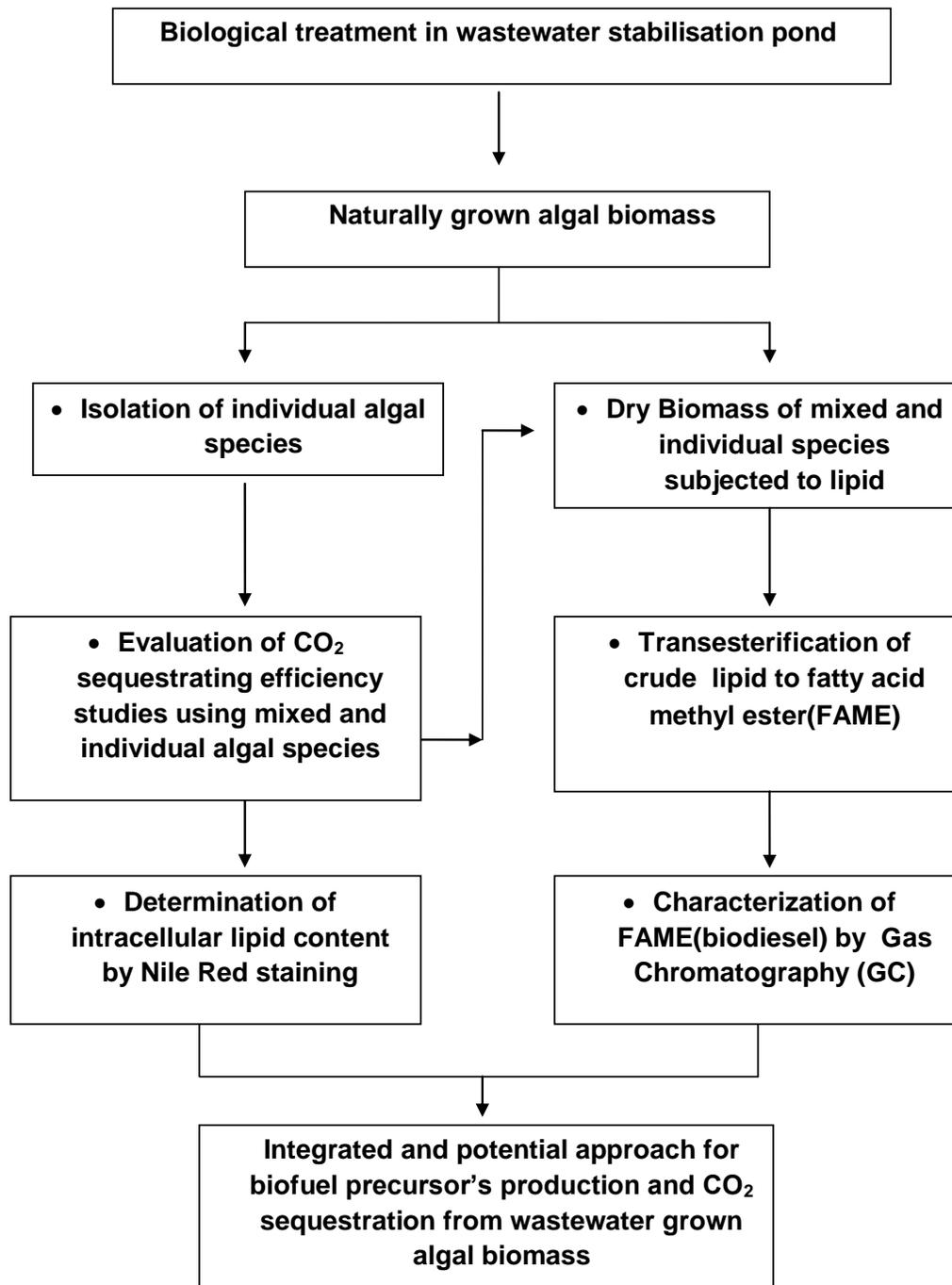
**Figure 4.** Stepwise analysis for integrated biofuel precursor production and CO<sub>2</sub> sequestration from algae biomass grown in wastewater.
