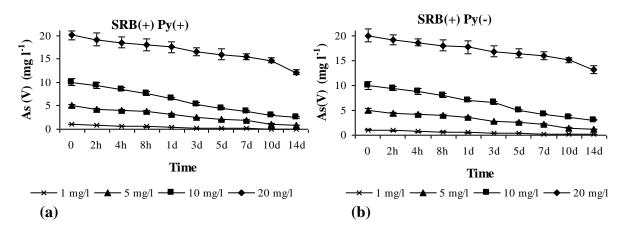
**Figure 11.** Changes in As(V) concentration as a function of time in the presence of: (a) polystyrene immobilised SRB (SRB(+) Py(-)) and (b) in the presence of planktonic SRB (SRB(+) Py(-)).
