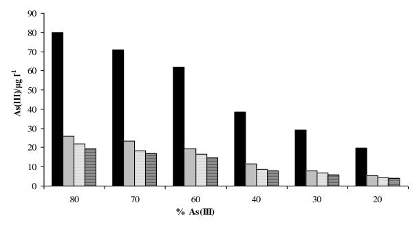
**Figure 13.** Changes in As(III) concentration when solutions containing various initial concentrations of this arsenic species in an As(III)-As(V) mixture were in contact with 0.1, 1 and 2 g/l  $MnO_2$  for 24 h at pH 6.9.
