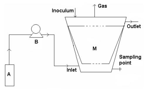
**Figure 2.** Bioreactor configuration: A – arsenic-contaminated water reservoir; B – peristaltic pump; M – support matrix within the inner channels.
