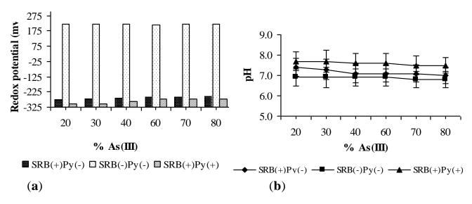
**Figure 6** Changes in (a) redox potential and (b) pH as a function of initial percentage of As(III) in a total arsenic concentration of 0.1 mg/l in the presence of SRB with polystyrene as support matrix (SRB(+) Py(+)), in the absence of SRB and polystyrene (SRB(-) Py(-)) and in the presence of planktonic SRB (SRB(+) Py(-)).
