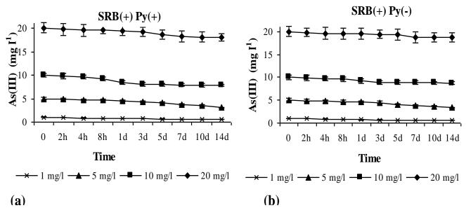
**Figure 10.** Changes in As(III) concentration as a function of time in the presence of: (a) polystyrene immobilised SRB (SRB(+) Py(+)) and (b) in the presence of planktonic SRB (SRB(+) Py(-)).
