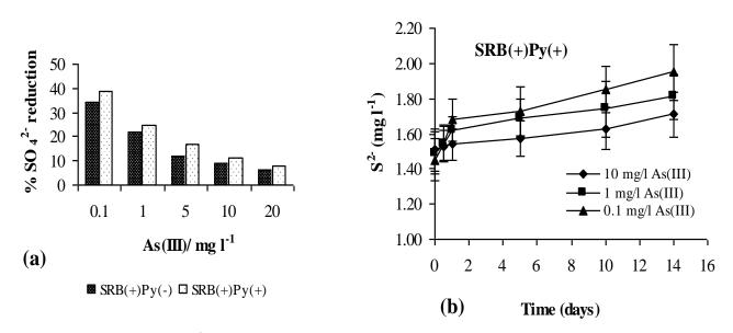
**Figure 7.** (a) Percentage of  $SO_4^{2^{\circ}}$  reduction as a function of As(III) concentration in the presence of polystyrene immobilised SRB (SRB(+) Py(+)) and in the presence of planktonic SRB (SRB(+) Py(-)); (b) Changes in S<sup>2-</sup> concentration as a function of time in the presence of polystyrene-immobilised SRB (SRB(+) Py(+)) growing in the presence of different As(III) levels.
