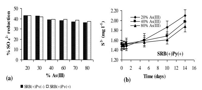
**Figure 9.** (a) Percentage of  $SO_4^{2-}$  reduction as a function of the percentage As(III) in a mixture of As(III) and As(V) (total arsenic = 0.1 mg/l) in the presence of polystyrene immobilised SRB (SRB(+) Py(+)) and in the presence of planktonic SRB (SRB(+) Py(-)). (b) Changes in S<sup>2-</sup> concentration as a function of time in the presence of polystyrene-immobilised SRB (SRB(+) Py(+)) growing in the presence of different As(III) and As(V) combinations.
