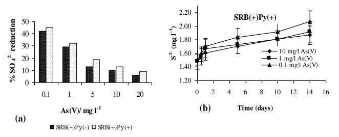
**Figure 8.** (a) Percentage of  $SO_4^{2^{\circ}}$  reduction as a function of As(V) concentration in the presence of polystyrene immobilised SRB (SRB(+) Py(+)) and in the presence of planktonic SRB (SRB(+) Py(-)). (b) Changes in S<sup>2-</sup> concentration as a function of time in the presence of polystyrene-immobilised SRB (SRB(+) Py(+)) growing in the presence of different As(V) levels.
