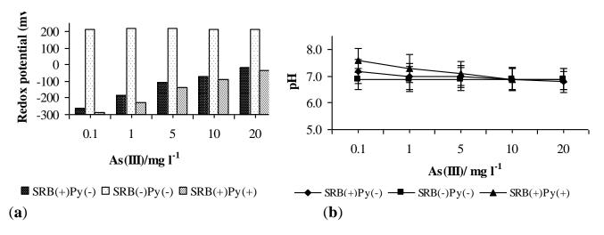
**Figure 4** Changes in (a) redox potential and (b) pH as a function of As(III) concentration in the presence of SRB with polystyrene as support matrix (SRB(+) Py(+)), in the absence of SRB and polystyrene (SRB(-) Py(-)) and in the presence of planktonic SRB (SRB(+) Py(-)).
