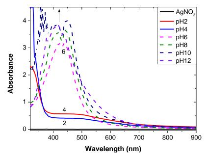
**Figure 4.** UV-Vis spectra of the variation of pH in *Ipomea batatas* leaf extract. Dash curves represent solutions diluted by 0.5.
