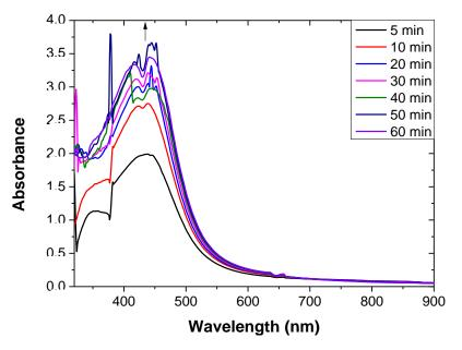
Figure 2. 60 min monitoring of the reaction between 10 mL of Ipomea batatas leaves extract and 50 mL AgNO $_3$  10<sup>-3</sup> M.
