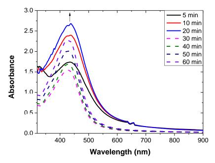
**Figure 1.** Monitoring 60 min of the reaction between 10 mL of *Chorcorus olitorus* leaves extract and 50 mL AgNO<sub>3</sub>  $10^{-3}$  M. Dash curves represent solutions diluted by 0.5 due to their maxima higher than the maximum 4.5 u.a."
