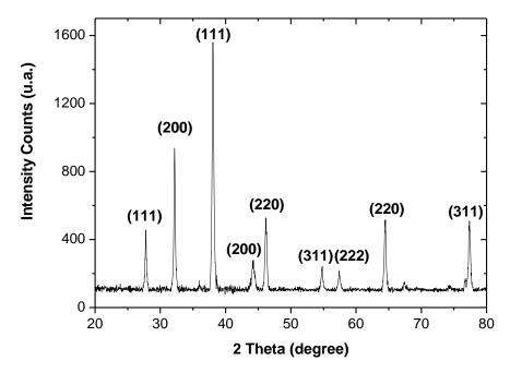
Figure 6. XRD pattern of the nanoparticles in Corchorus olitorus.
