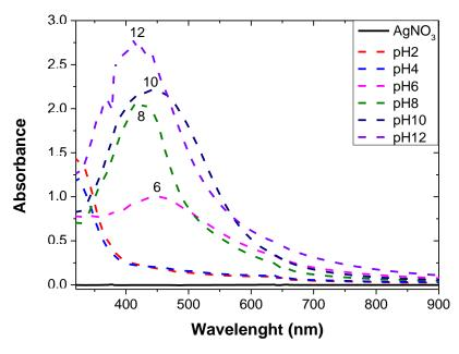
**Figure 3.** UV-Vis spectra of the variation of pH in *Corchorus olitorus* leaf extract. Dash curves represent solutions diluted by 0.5.
