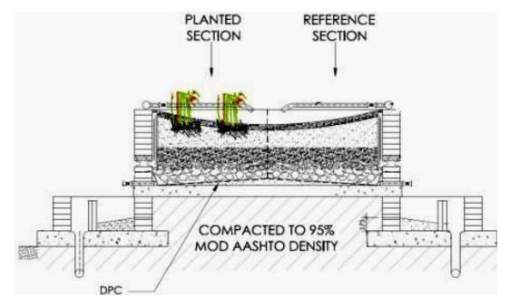
**Figure 2.** Cross section of the multi-engineerd system. The plants are planted in such a way that they are evenly distributed across the test section of the wetland. The layout of plants in the wetland medium can be seen in Figure 1. Species of the plants used are *Phragmites australis*.
