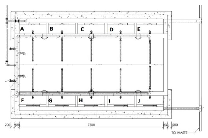
Figure 1. Schematic representation of a multi-designed wetland system in Durban.
