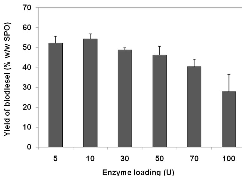
**Figure 4.** Effect of enzyme loading on biodiesel production from sludge palm oil (SPO) using locally produced *Candida cylindracea* lipase.
