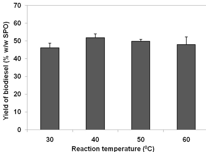
**Figure 5.** Effect of reaction temperature on biodiesel production from sludge palm oil (SPO) using locally produced *Candida cylindracea* lipase.
