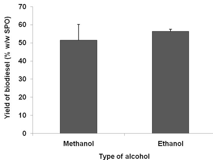
Figure 2. Effect of methanol and ethanol on biodiesel production from sludge palm oil (SPO) using locally produced *Candida cylindracea* lipase.
