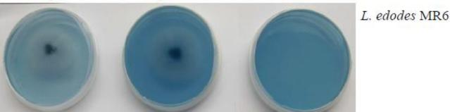
Figure 1. Decolourization of media containing 200 mg/L RBBR by local isolates P. ostreatus MR3 and L.edodes MR6. Controls without inoculums.
