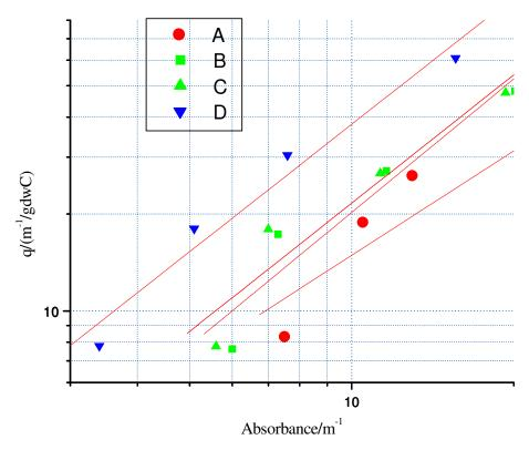
**Figure 4.** Freundlich adsorption isotherm lines for  $UV_{254}$  of the GAC samples at different heights of the biofilter. A, B, C and D: BAC samples taken from different heights of the biofiler; at 0.25, 0.45, 0.65 and 0.85 m, respectively.
