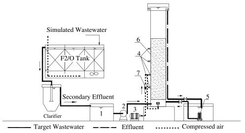
1 Storage tank 2 Metering pump 3 Air comprasspr 4 Sampling ports 5 Backwash pump 6 UABACF 7 Gas flowmeter
