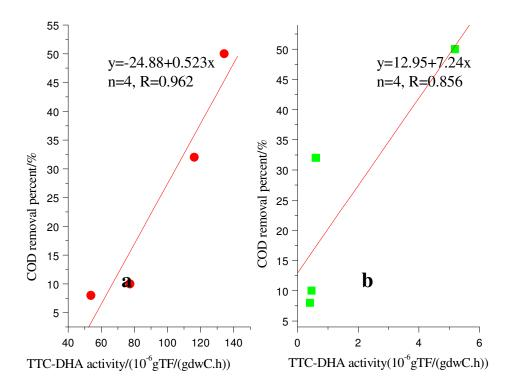
**Figure 3.** Correlations between COD removal proportions and bioactivities at different height sections of the biofilter: **a.** TTC-DHA activities determined in modified way. **b.** TTC-DHA activities determined in conventional way.
