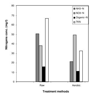
**Figure 5.** Results of Nitrogens concentration of raw and treated sludge.
