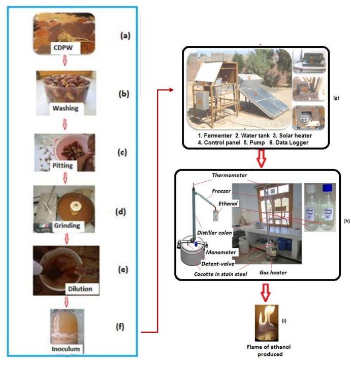
Figure 2. Bioethanol generation process.
