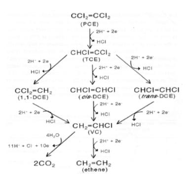
Figure 1. Proposed pathway for biological transformation of chlorinated ethenes (Maymo-Gatelle et al., 1997).
