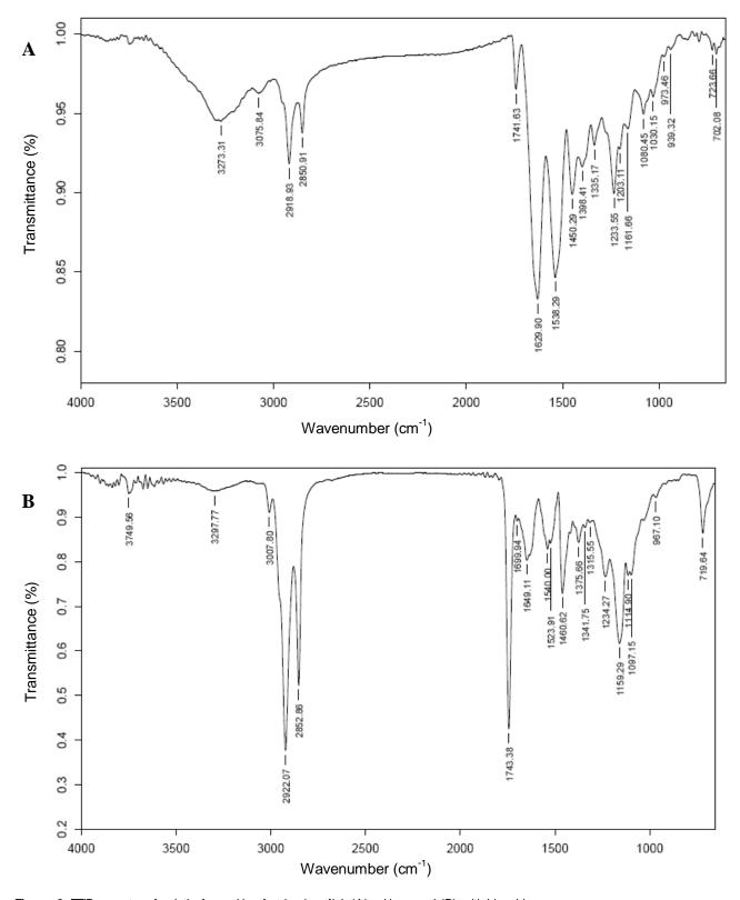
Figure 2. FTIR spectra of gelatin from skin of striped catfish (A) with no and (B) with bleaching.
