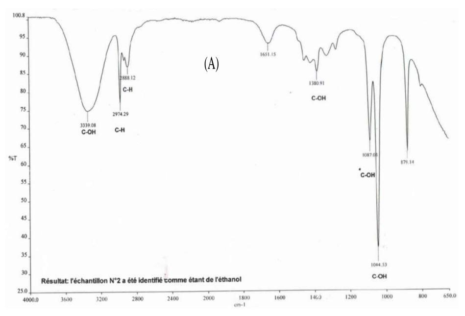
Figure 9. Infra-Red Spectra of the bioethanol produced. (A) Teggaza; (B) Lebghel.
