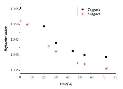
Figure 7. Refractive index during the fermentation process.
