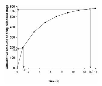
**Figure 1.** Model of dissolution profile of the multiunit dose tablets showing the prompt release dose ( $m_p=200~mg$ ) and time to attain it  $t_p$  (1 h), the maximum release ( $m_\infty=600~mg$ ) at  $t_\infty=12~h$ .
