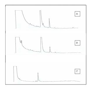
**Figure 3.** GC analysis of acid-line and alkali-line composite effluent before fungal treatment (A), after fungal treatment under non-shaking conditions (B) and under shaking conditions (C).
