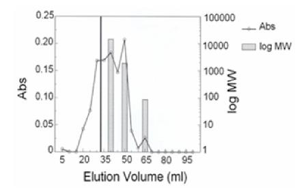
**Figure 2.** Molecular weight distribution of alkali-line effluents (Note: Those with elution volumes less than 32 ml have molecular weight greater than 30 000).
