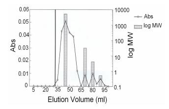
**Figure 1.** Molecular weight distribution of acid-line effluents (Note: Those with elution volumes less than 32 ml have molecular weight greater than 30 000).
