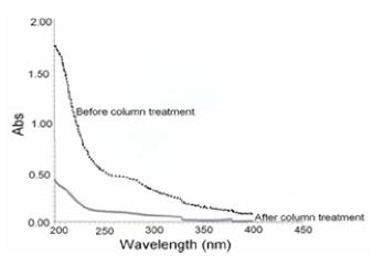
Figure 4. UV scans of acid-line and alkali-line bleachery effluent sample before and after column treatment.
