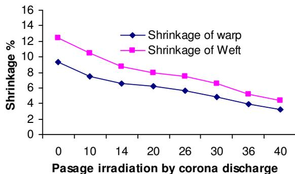
Figure 3. The shrinkage amount in warp and weft fibers in 4 washing cycle.
