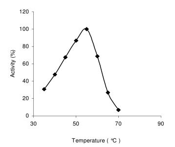
**Figure 7.** Effect of temperature on *Periplaneta americana*  $\alpha$ -amylase. Reaction mixtures containing 100  $\mu$ l of enzyme solution, 100  $\mu$ l of 20 mM acetate buffer (pH 5.6) and 100  $\mu$ l of 1% soluble starch were incubated at various temperatures (35 – 70 °C) for 20 min and the amount of reducing sugars produced was determined by the DNS method.
