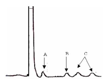
**Figure 12.** Chromatogram of soluble starch degradation products. Column connected: supercosyl LC-NH<sub>2</sub> 5 µm (0.46 x 25 cm); mobile phase: water-acetonitrile (25/75, v/v); flow rate: 0.75 ml/min; peak A: xylose (internal standard); peak B: maltose; peak C: maltodextrin. The experiments were performed with 0.58 U of  $\alpha$ -amylase.
