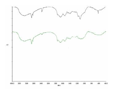
Figure 5. IR Spectra of pullulan produced by *Aureobasidium pullulans* from matured coconut water (top) and coconut milk (bottom).
