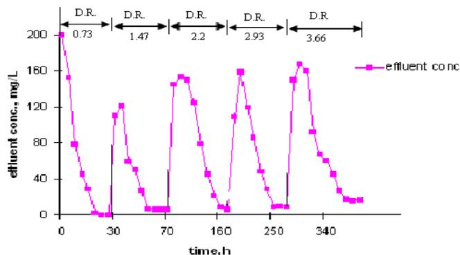
**Figure 6.** Effect of dilution rate on steady state effluent concentration.
