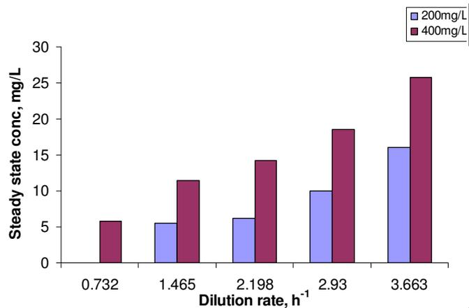
**Figure 7.** Comparison of steady state effluent phenol concentration for different dilution rate at 200 and 400 mg/L influent phenol concentration.
