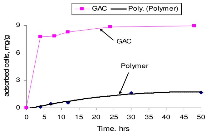
Figure 2. Plot of time against Immobilization of cells/ gm of solid.
