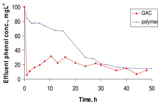
**Figure 4.** Effluent phenol concentration during startup period (influent phenol conc. = 100 mg/L; dilution rate = 2.2 h<sup>-1</sup>).
