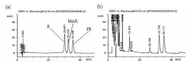
**Figure 3.** HPLC traces of standard samples and the reaction mixture using *M. morganii* CMCC(B) 49208 for the bioconversion of MAK to (1S, 2S) -ephedrine. (a) standard samples of (1R, 2S) -ephedrine (E), (1S, 2S) -ephedrine (PE), and MAK; (b) chemicals in the reaction mixture using *M. morganii* CMCC(B) 49208.
