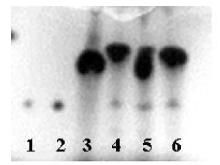
**Figure 2**. Screening of *M. morganii* strains for the bioconversion of MAK to ephedrine by TLC. Lane 1. (1R,2S) -ephedrine; lane 2. (1S,2S) -ephedrine; lane 3. final reaction mixture using *M. morganii* CMCC(B)49214; lane 4. CMCC(B)49209; lane 5. CMCC(B)49208; and lane 6. CMCC(B)49203.
