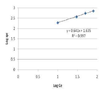
Figure 6. Freundlich isotherm for the sorption of basic dye  $30 \,^\circ C$  using bamboo as absorbent.
