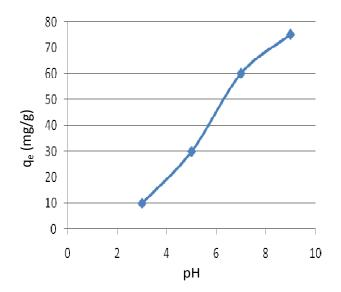
**Figure 2.** Effect of pH on the sorption of basic dye at 30 °C using bamboo as absorbent.
