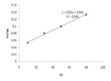
Figure 5. Langmuir isotherm for the sorption of basic dye at 30 ℃ using bamboo as absorbent.
