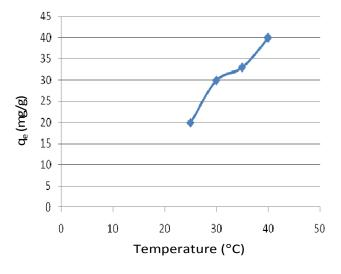
Figure 3. Effect of temperature on the sorption of basic dye at 30  $^\circ\!\!C$  using bamboo as absorbent.
