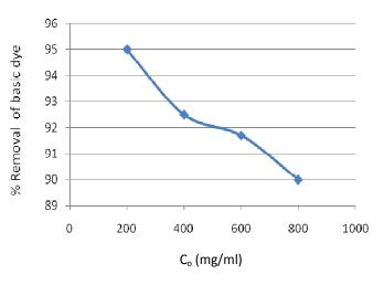
Figure 4. Effect of initial dye concentration on its removal using bamboo as absorbent.
