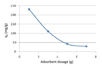
Figure 1. Effect adsorbent (bamboo) dosage on the sorption of basic dye at 30  $^{\circ}\!C.$
