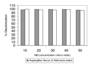
Figure 1. Efect of dye concentration on % decolorization of malachite green. Incubation period: 6 days.
