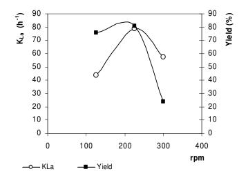
**Figure 3.** Volumetric mass transfer coefficient for  $O_2$ ,  $h^{-1}$ , and yield, atdifferent agitation rates.
