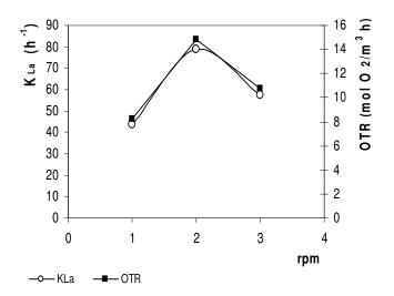
**Figure 1.** Volumetric mass transfer coefficient for  $O_2$ ,  $h^{-1}$ , and OTR, mol m<sup>-3</sup>  $h^{-1}$ , at different agitation rates (1, 2 and 3 on the x-axis represents 126, 226 and 300 rpm, respectively).
