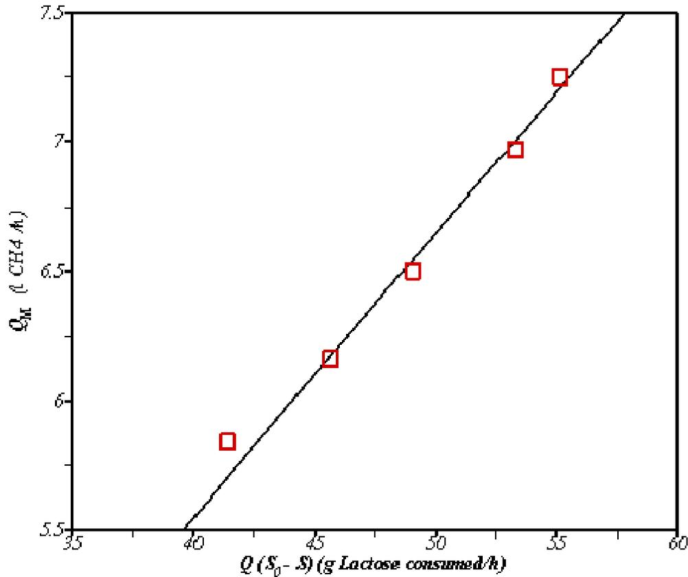
Figure 6. Methane production with respect to utilized substrate.
