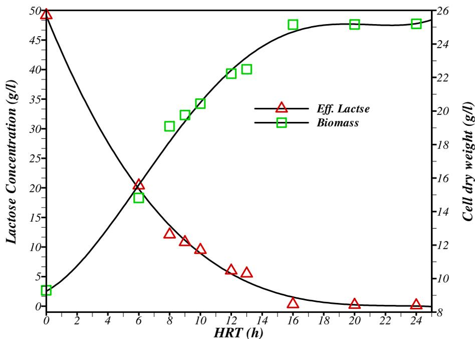
**Figure 2.** Lactose consumption profile and cell growth curve with respect to HRT.
