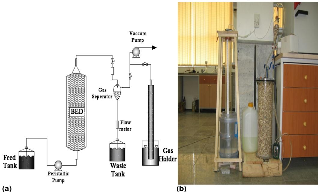
**Figure 1.** Schematic diagram of experimental set up: a. UAPB flow diagram. b. Fabricated pilot scale of the bioreactor.
