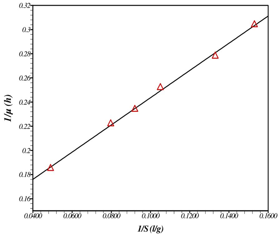
Figure 4. Linearized double-reciprocal plot of the specific growth and substrate.
