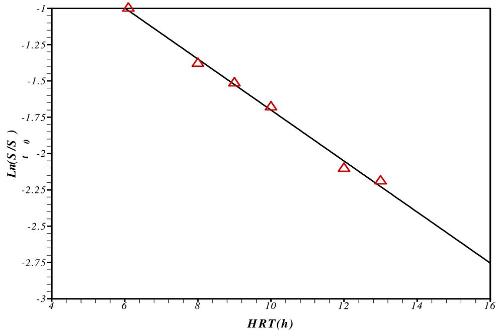
Figure 3. Logarithmic rate model for substrate utilization.
