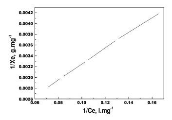
Figure 8. Langmuir plot for Pb<sup>2+</sup> ions adsorption onto PACI.
