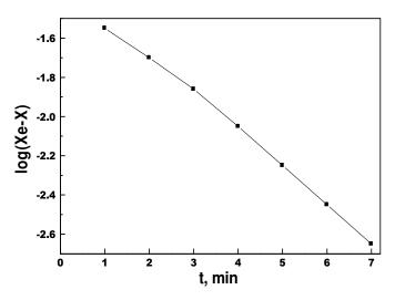
Figure 4. Plot of log (X<sub>e</sub>-X) versus stirring time for  $Pb^{2+}$  ions adsorption onto 100 mg.l<sup>-1</sup> PACI.
