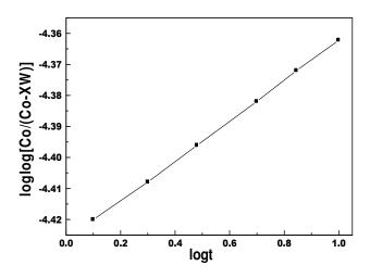
Figure 3. Plot of log log  $[C_o/(C_o - XW)]$  versus log t for the adsorption of Pb<sup>2+</sup> ions by 100 mg.l<sup>-1</sup> PAC at pH 7.
