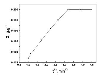
**Figure 2.** Plot of the amount of  $Pb^{2+}$  ions adsorbed onto 100 mg. $I^{-1}$  PACI versus square root of time at pH 7.
