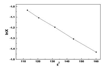
Figure 10. Dubinin-Radushkevich (D-R) plot for  $Pb^{2+}$  ions adsorption on to PACI.
