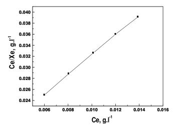
Figure 9. Second Langmuir plot for  $Pb^{2+}$  ions onto 100 mg.l<sup>-1</sup> of PACI.
