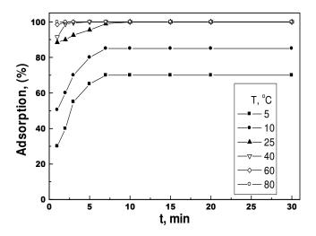
**Figure 6.** Adsorption of 20 mg.l<sup>-1</sup> of Pb<sup>2+</sup> ions by 100 mg.l<sup>-1</sup> PACI at different temperatures and varying stirring times at pH 7.
