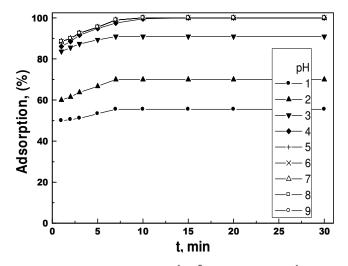
Figure 5. Adsorption of 20 mg. $l^{-1}$  Pb<sup>2+</sup> ions by 100 mg. $l^{-1}$  PACI versus stirring time and pH.
