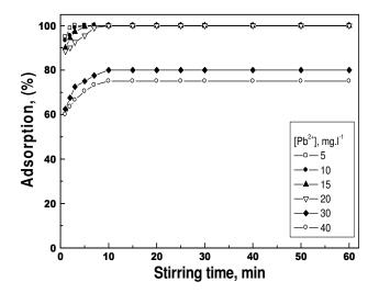
**Figure 1.** Influence of stirring time on the adsorption of different Pb<sup>2+</sup> ion concentrations onto 100 mg.I<sup>-1</sup> PACI at pH 7.
